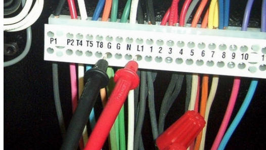
Figure 6: Note the black lead on ground and the red lead measuring voltage
